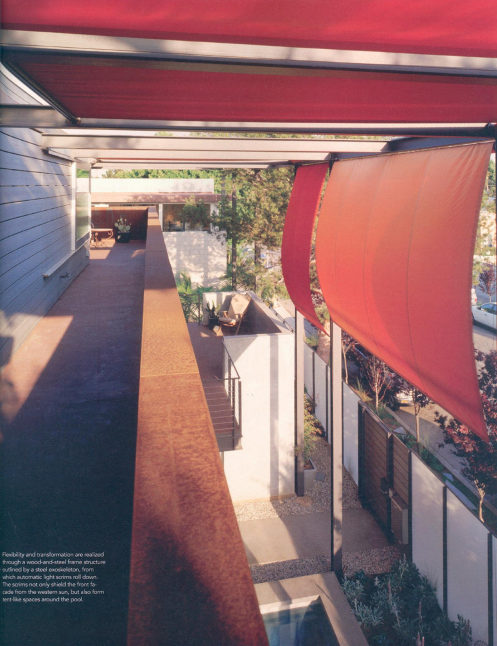
Flexibility and transformation are realized through a wood-and-steel frame structure outlined by a steel exoskeleton, from which automatic light scrims roll down. The scrims not only shield the front facade from the western sun, but also form tent-like spaces around the pool.
